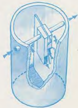
Septic tanks may be constructed of glass fibre, thermoplastics or precast concrete.
